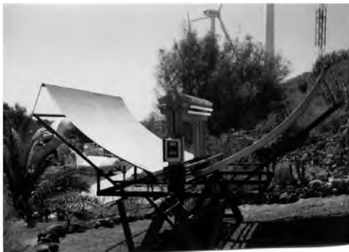
Fig. 2. The follow-up system with concentration system, ITER Tenerife, [phot. Grażyna Frydrychowicz-Jastrzębska]
