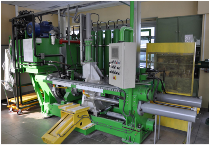
Fig. 7. Backward extrusion 5 MN capacity hydraulic press – type PH-LR 500
