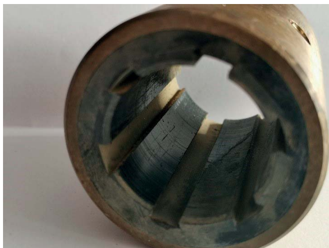
Fig. 5. The PTFE sliding bush (B)
