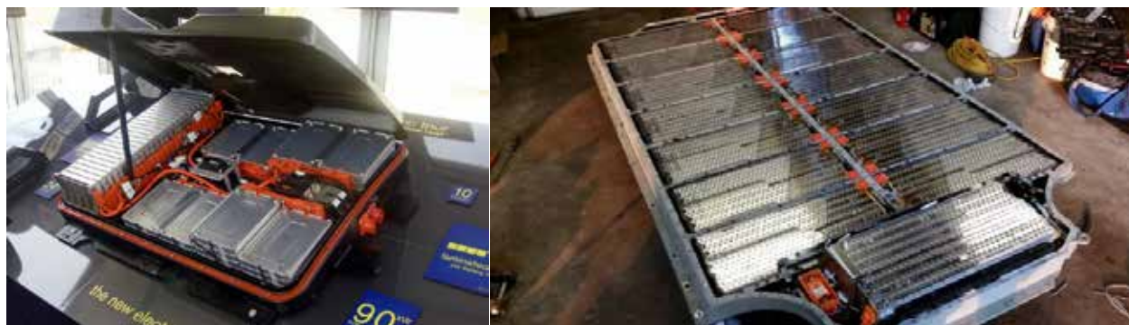
a) accumulator battery of Nissan Leaf; b) accumulator battery of Tesla Model S
