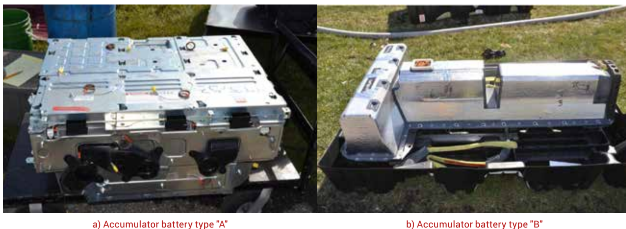
Figure 8. An example of accumulator batteries for carrying out full-scale fire experiments [12]
