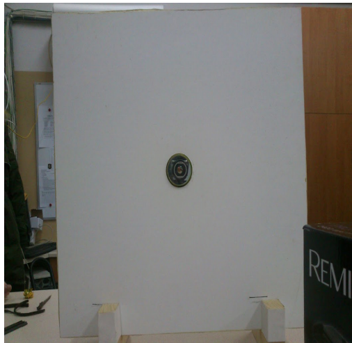
Fig. 2. The insulation board with the sample holder
