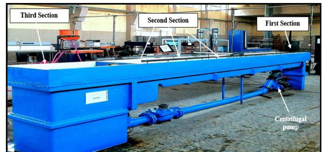
Fig. 2. The laboratory flume; source: own elaboration
