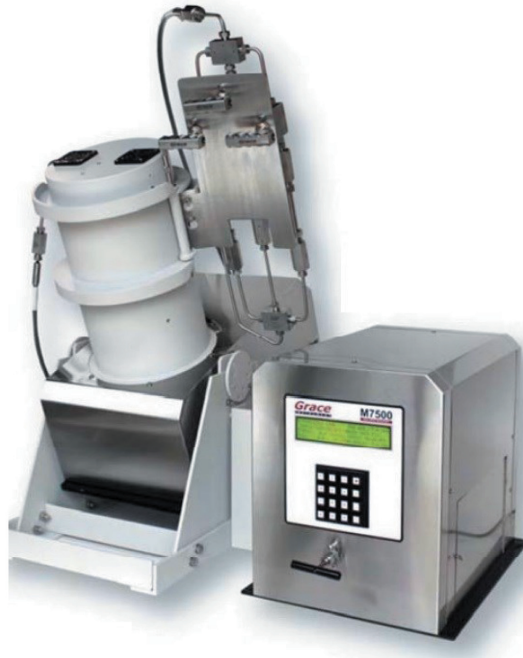
Fig. 8. Grace Sagging Tester M8500 Ultra HPHT [9]
