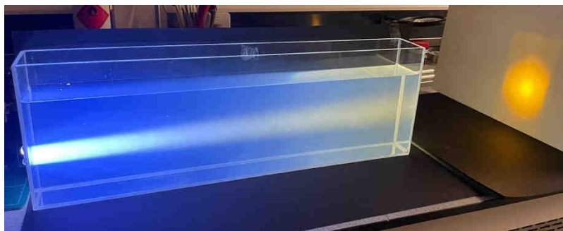
Fig. 31. Scattering of light by colloidal sulphur (courtesy of Andres Tretiakov)
