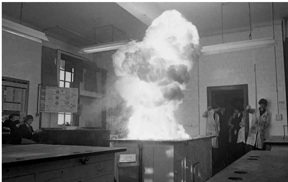
Fig. 24. Reaction between sulphur and excess zinc
