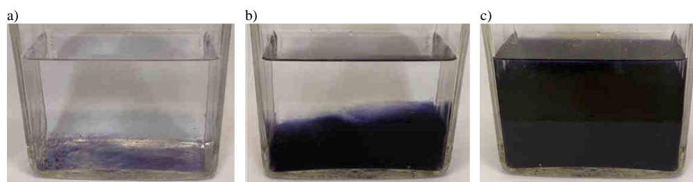
Fig. 33. Iodine clock reaction, showing the gradual appearance after of the blue-black colour in an unstirred iodine clock reaction mixture: a) 20 seconds, b) 30 seconds, c) 45 seconds
