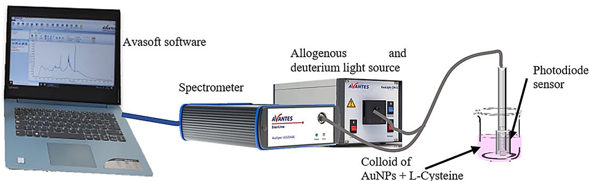
Figure 3. Sequence diagram for colloid characterization of functionalized AuNPs
