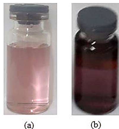
Figure 13. (a) AuNPs + L-Cysteine and (b) AuNPs + L-Cysteine with analyte ion interactions
