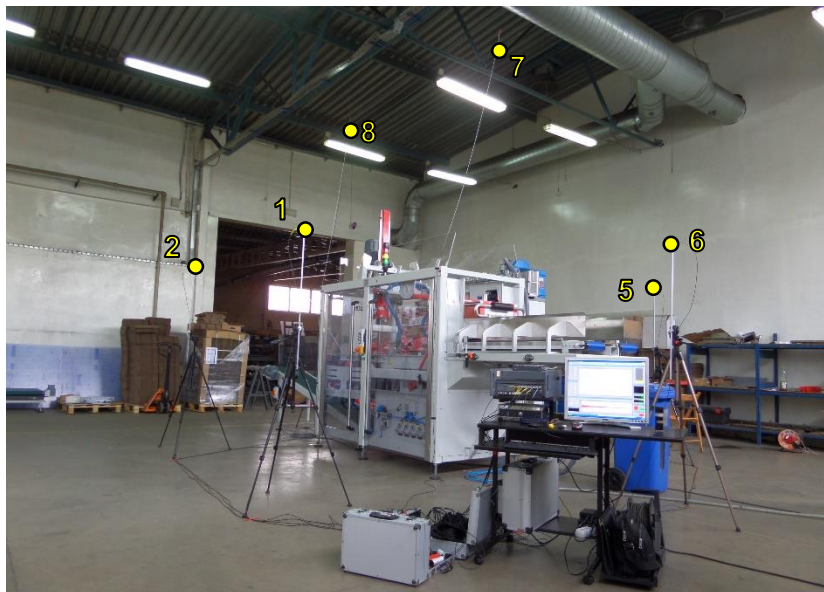
Figure 4. View of the tested object - FTHT 6 former, after preparation for sound pressure measurements (measurement points 3 and 4 are behind the former)
