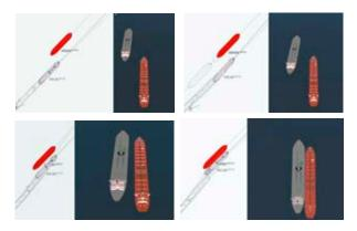
Figure 4. Service ship approaching STBL on the parallel course with the sufficient side distance, approaching parallel and adjusting speed with course 1° smaller than she goes
