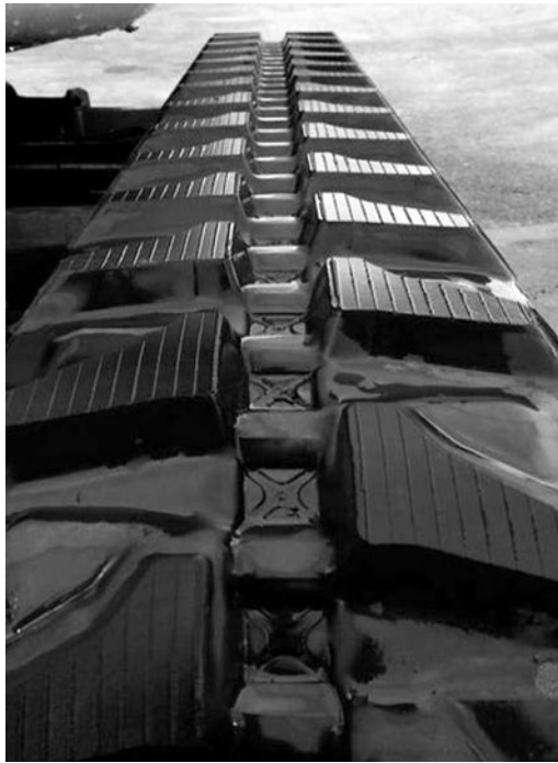
Fig. 6. The elastomeric track No. 1, the non-operated specimen. There are no cracks and damages at its surface, the tread edges are sharp and the segment walls are uniform, Visible remnants of the production process in the form of linear shoulders
