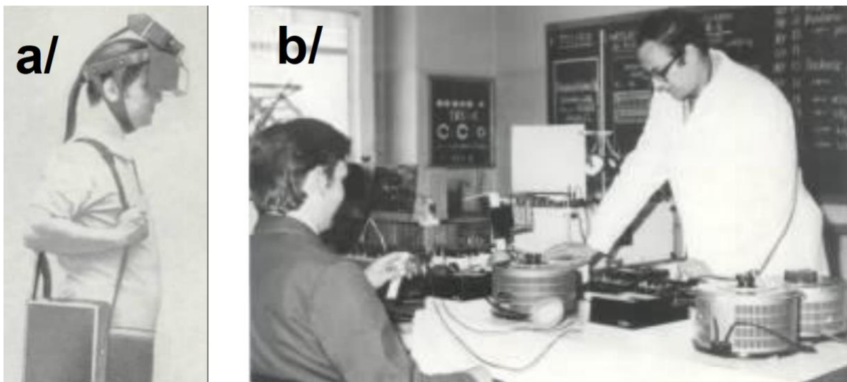
Fig. 9 Polish innovations: a) Elektroftalm – a device for transmitting visual information through vibrations stimulating the skin of the forehead, b) Director of the Bureau of Aviation Electronics Designs in Poznań Dr Mieczysław Cenin during the doctoral examination of the pilot's response time at the electro-touch transmission of visual information to the brain (3 times faster than sight) in 1975.
