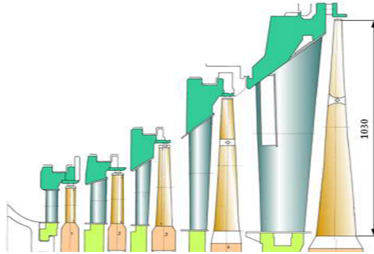
Figure 1: Longitudinal section of the low-pressure cylinder (LPC) of the K-220-44-3 series turbine.
