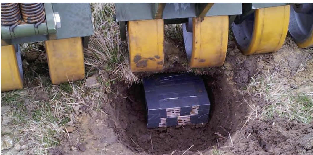
Fig. 3. Explosive charges placed under the wheel of mine flail
