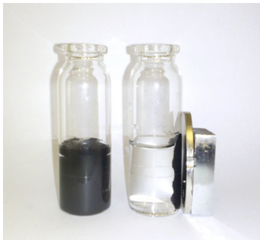
Figure 3. Photograph of magnetic separation of Fe@G from the aqueous solution with a permanent magnet
