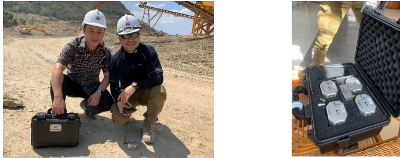
Fig. 2. Seismograph for monitoring blast-induced ground vibration in the Thuong Tan III quarry.
