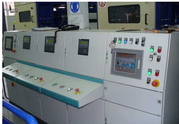
Fig. 22. The components of stitched non-woven fabric production line a) final needlepunching unit, b) control desk
