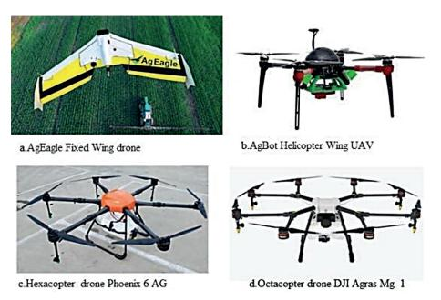
Figure 6. Types of UAV's used in Agriculture fields
