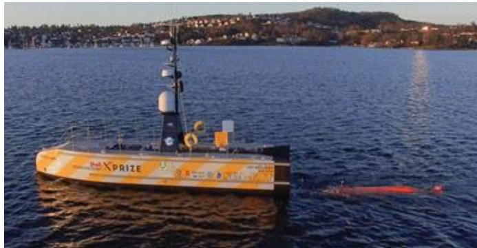
Fig. 7. Aerial view of SEA-KIT during HUGIN retrieval operations. (credit: Lew Abramson, Inner Space Center)
