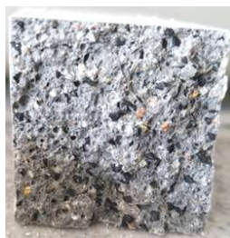
Fig. 4. 4x4 cm fracture of the GK-D cement mortar beam after bending strength test with visible black SBR-D rubber granules
