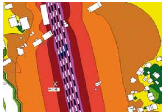
Figure 3. Map L_{day} calculated for a measurement point with SRM II [4]. Notes. L_{day} —A-weighted long-term average sound level as defined in Standard No. ISO 1996-2:2007 [37], determined over all day periods of a year.
