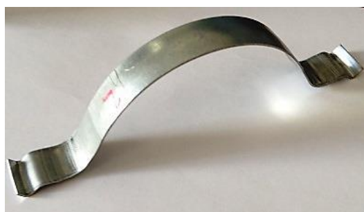
Fig. 4. Formed sample for springback analysis
