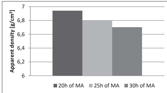
Fig. 6. Influence of milling time on apparent density of Cu-10 wt.% TiN
