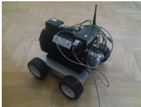
Fig. 1. The mobile platform with the onboard computer and essential sensors installed
