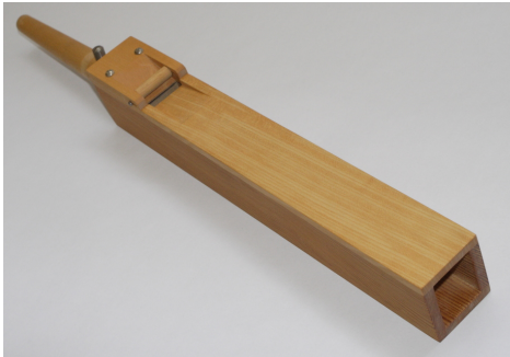
Fig. 9. A real-world example of an organ pipe for which the difference between length correction predictions 0.61a and 0.72a should be clearly audible.
