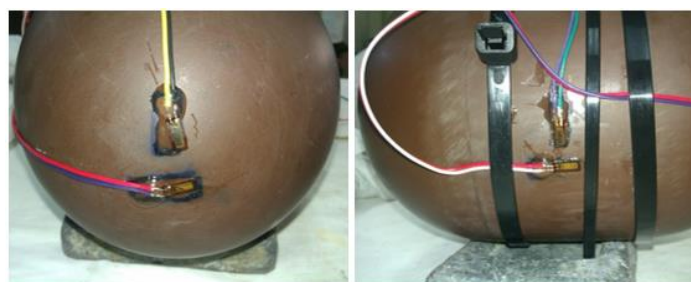
Fig. 8. Strain measurements system – examples of the measurement points on the spherical (left) and cylindrical part (right)
