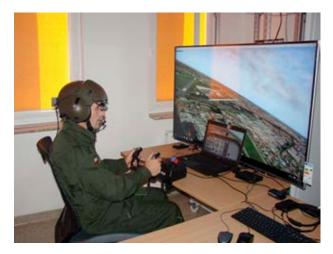
Figure 15. The flight simulator with a helmet-mounted flight parameter imaging system (AFIT)
