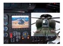
Figure 8. Imaging in daylight from the TOPLITE observation-targeting head displayed on the head monitor for the second pilot-operator of a W3PL "Gluszec" helicopter (AFIT)
