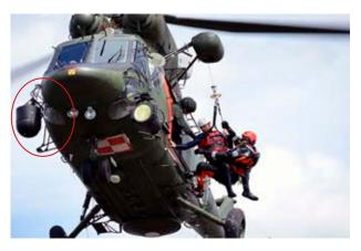
Figure 2. W3WA helicopter adapted for the needs of search and rescue missions with an installed winch (Wikipedia.pl)
