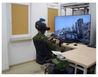
Figure 16. Simulated flight in the area in which the survivor is present, with the use of a helmet-mounted information imaging (AFIT)
