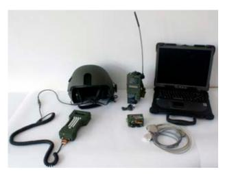
Figure 10. Headphone circuit of a crew commander or pilot-operator of a Mi17 helicopter with an integrated communication system (AFIT)
