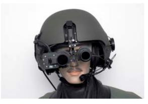
Figure 12. NWN1 night-time display of the SWPL1 "Cyklop" and night vision goggles mounted on the THL5 helmet (AFIT)
