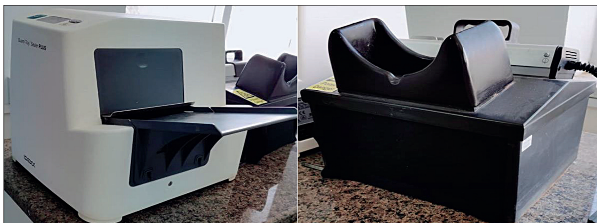
Figure 1. (a) The quanti-tray sealer, (b) UV lamp cabinet
