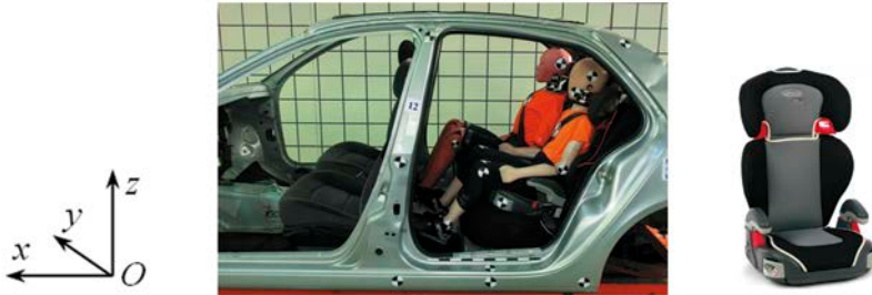
Fig. 4. Test dummies in the car body and a child safety seat for the P10 dummy
