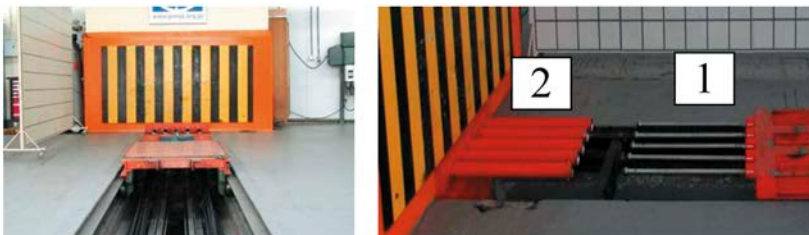
Fig. 3. Trolley and braking system of the PIMOT measuring stand for crash tests
