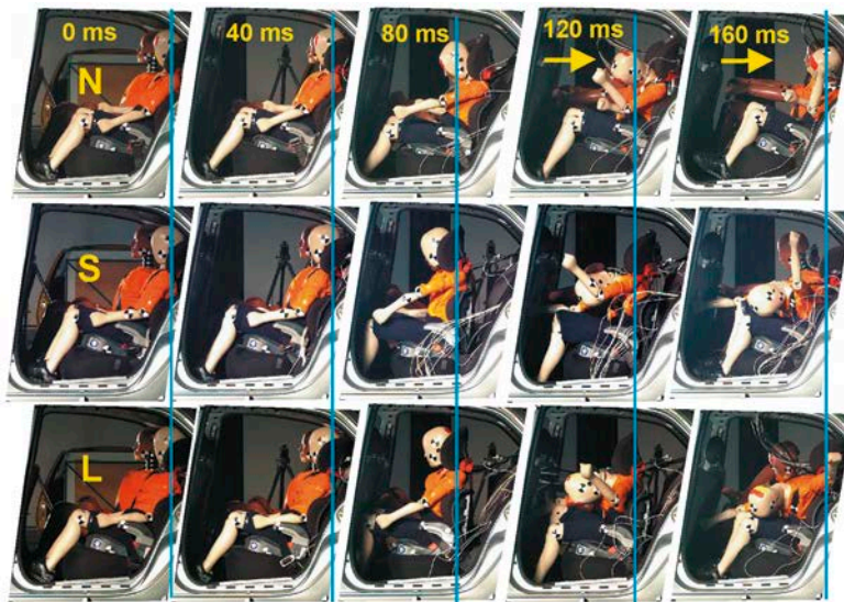
Fig. 12. Displacements of the P10 dummy at the N, S, and L tests (the vertical lines were drawn through a mark on the dummy's head at the N test; arrows indicate the direction of dummy's movement at the N test)
