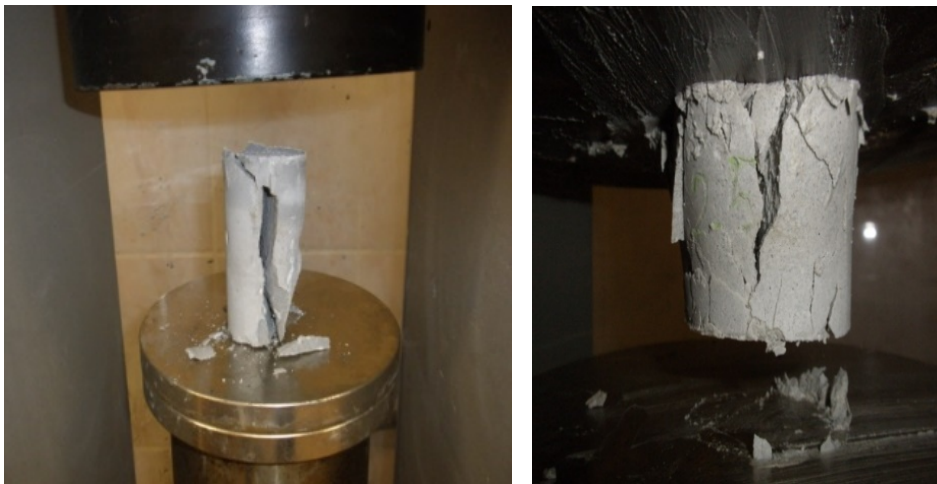
Fig. 11. Examples of samples after compressive strength tests
