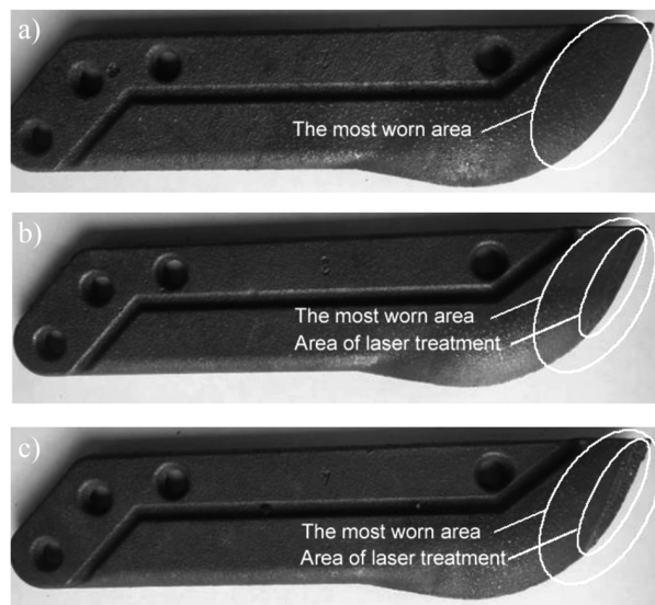
Fig. 15. The coultter flap (after wear test): without laser treatment (a), after laser alloying with boron (b) and after laser alloying with mixture of boron and chromium (c)
