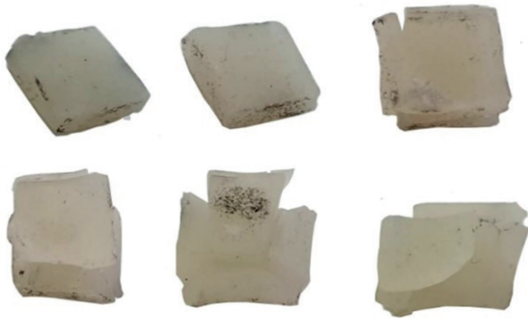
Fig. 2. Samples after reaching the swelling equilibrium state, from left: PLA/ENR vulcanizates: 90/10, 80/20, 70/30, 60/40, 60/40_DDSQ-eter-4OH, 60/40_DDSQ-eter-4OH_5
