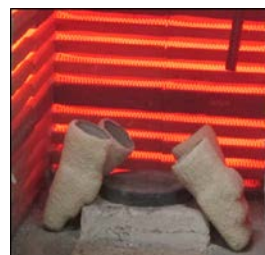
Fig. 3. Firing of moulds in resistance heating furnace
