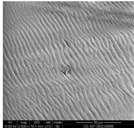
**Fig. 4. The surface of PE-UHMW cup after the test**
