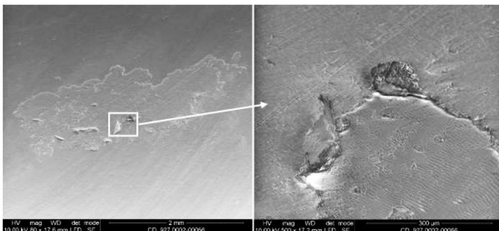
**Fig. 6. SEM micrograph of worn surface of UHMWPE insert, showing micro-delamination**
