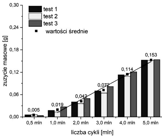
**Fig. 3. Mass loss of polyethylene cup taking into account control group**
