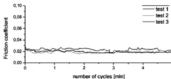
**Fig. 2. Friction coefficient curve for SBT simulator tests 01.2**
