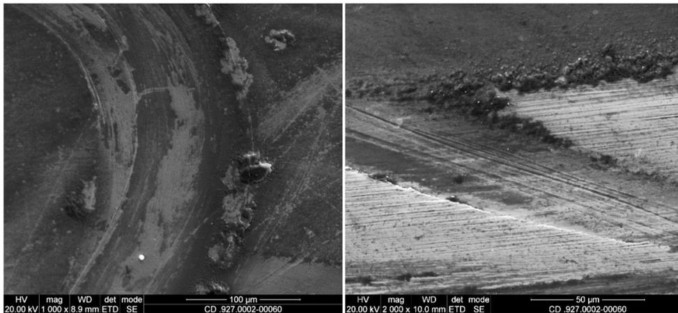
**Fig. 5. Morphology of head friction surface**
