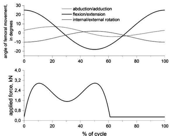
**Fig. 1. Graphs of variability over time: a) angular movements of femoral component, b) loading force values**
