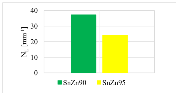
Fig. 5. Estimator of relative area ( N_L ) of ( \alpha -Zn+ \beta -Sn) eutectic precipitates in the examined binary alloys with high Zn content
