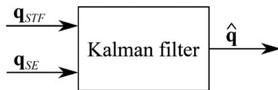
Fig. 5. Linear Kalman filter estimating attitude quaternion
