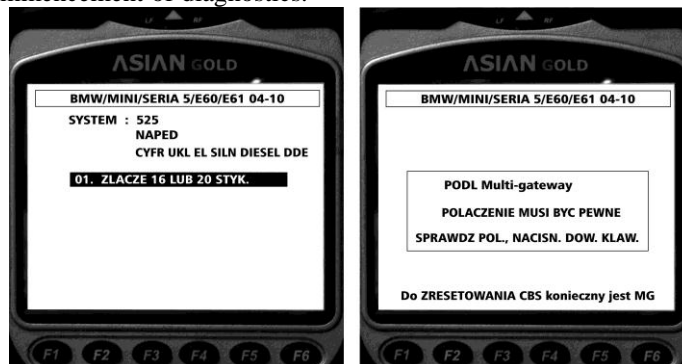
Fig. 7. Tester screens: choice of cable type (on the left), diagnosis effect (on the right)
