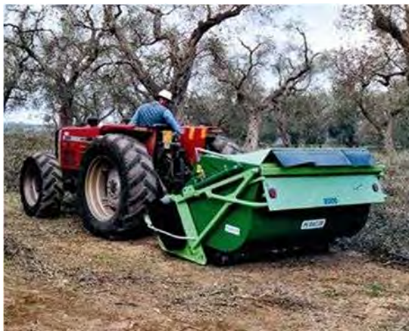
Figure 8. Flail mower collectors of wood biomass
