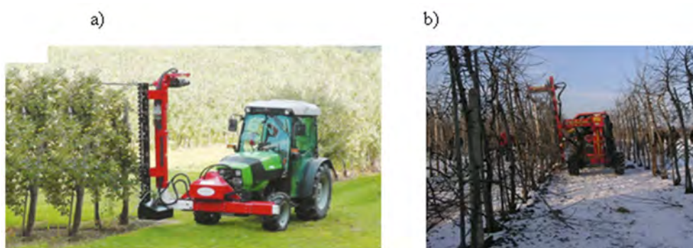
Figure 5. Pruning machine being operated in an apple orchard: a) blade pruning machine, b) disc pruning machine
