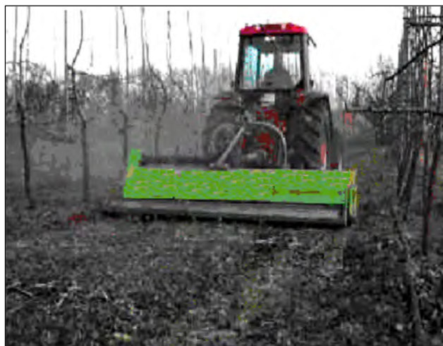
Figure 6. Hammer shredder being operated in an orchard
