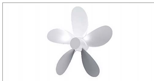
Fig. 2. JBC propeller geometry for case study “propeller open-water simulation”
