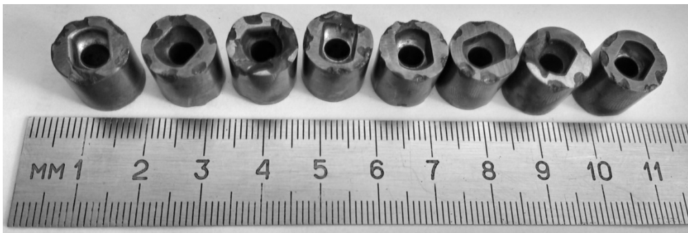
Fig. 5. Defects of cylindrical cutting tools
