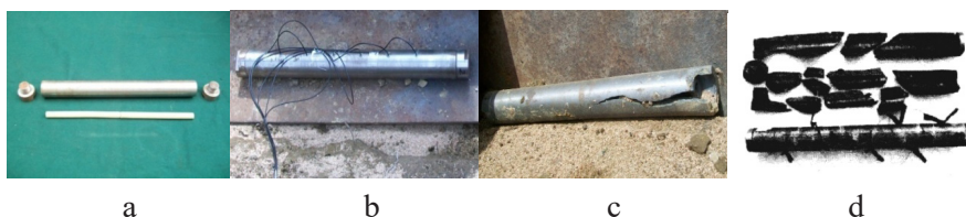
Figure 5. Actual test photographs of the DDT test: (a) DDT tube and propellant; (b) Test set up; (c) No detonation; (d) Detonation [13]
