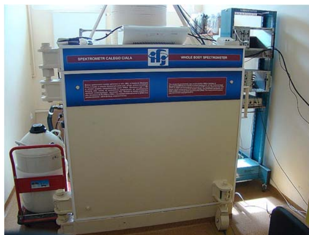
Fig. 2. A general view of the spectrometer with closed doors. Visible are also: a dewar of \text{LN}_2 refilling the system (left) and NIM electronics modules (right), ventilation system (on the top of the shield).
