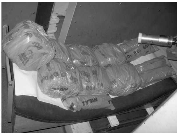
Fig. 4. A calibration phantom SICa-1 during preparation for measurements in the whole-body spectrometer, lying on the bed in extended position.
