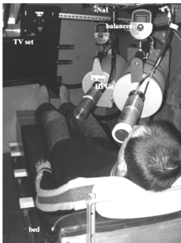
Fig. 3. A view of inside of the spectrometer prepared for measurement with a patient lying on the bed, visible: are the bed, two germanium detectors, the balances on the struts and TV. The NaI detector is moved upward, into the shield and only part of it can be noticed on the top of the picture.
