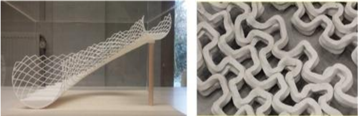
Fig. 4 Elaborate shapes of 3D printed concrete elements 34
