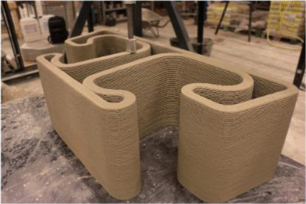
Fig. 3 Concrete element printed with inner empty spaces 33
