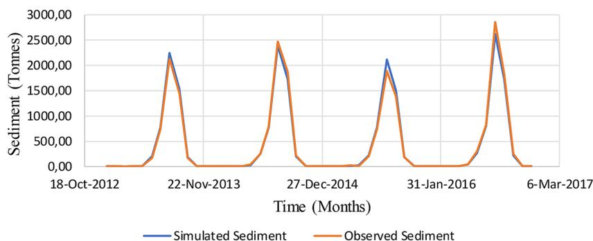
**Figure 8.** Computed sediment and observed sediment load during validation
