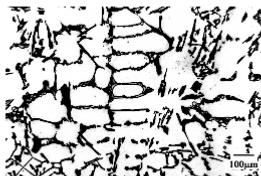
Fig. 4. Microstructure of AlSi8Cu2Mn alloy with EMF effect (B = 0.1 T, mag. 100x)
