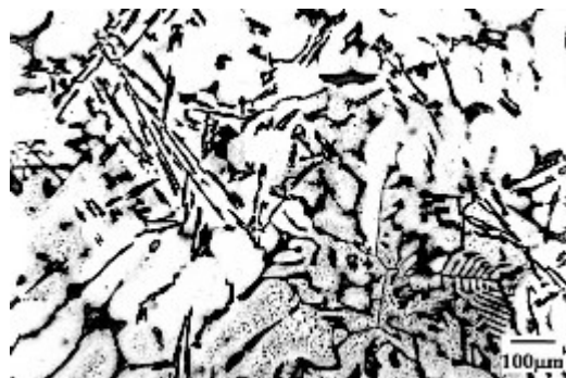
Fig. 3. Microstructure of AlSi8Cu2Mn alloy without EMF effect (mag. 100x)
