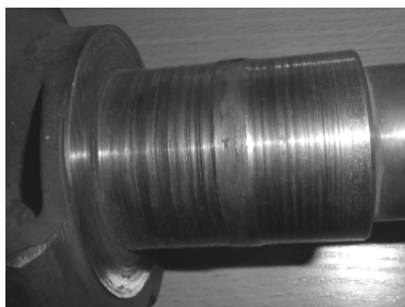
Fig. 1. Worn crankshaft journal with a trace of seizure
