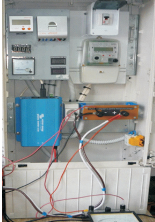
Fig. 1. Laboratory test stand for testing the processes of diagnosing low-capacity solar power station equipment (courtesy: S. Duer)
