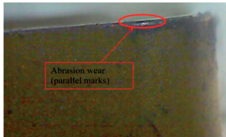
Fig. 8. Images of flank wear for tool with micro-channel
