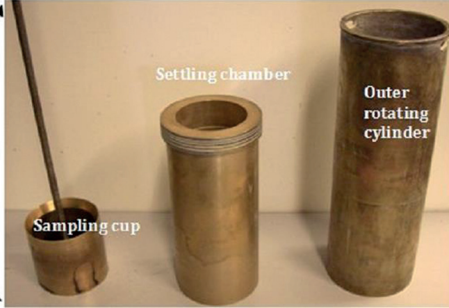
Fig. 4. Measuring system used in direct weight measurement method: a) measuring system; b) elements of measuring system: sampling cup where settling solids are collected, settling chamber, and outer rotating cylinder [4]
